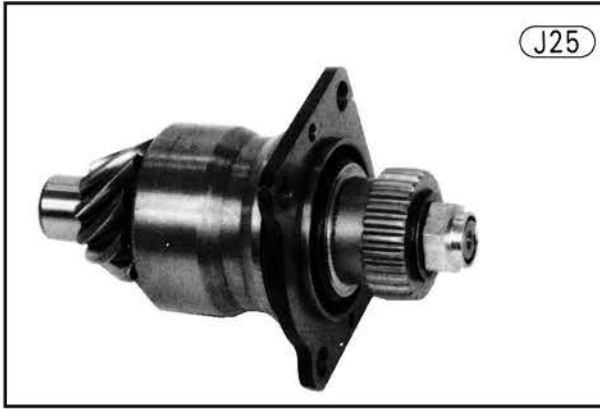
A. Check splined portion.
