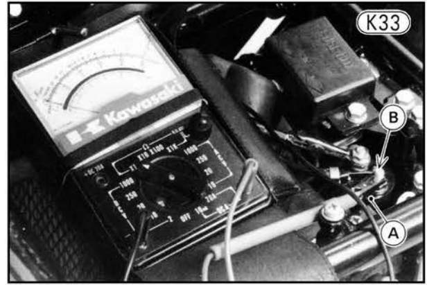
A. Starter Relay B. Disconnect the lead to the starter motor.
