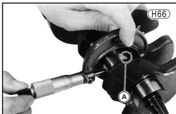
A. Avoid the oil hole for measurement.
